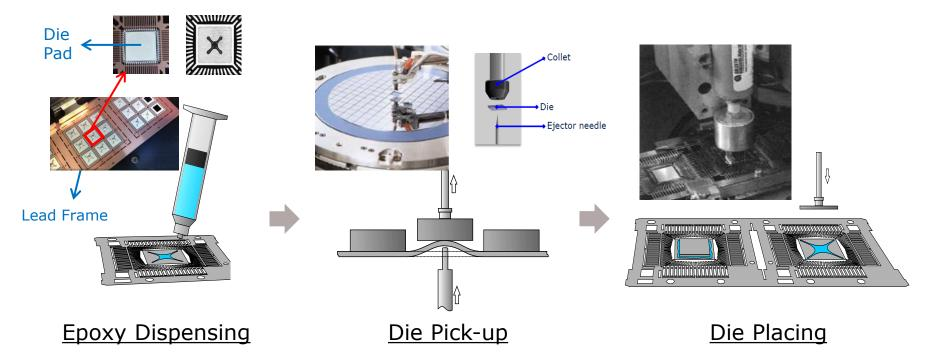
> Epoxy or solder is dispensed in the die flag area of the lead frame in a specified pattern (usually star) followed by a pick and place process that removes the die from the tape carrier and places it over the dispensed epoxy.
