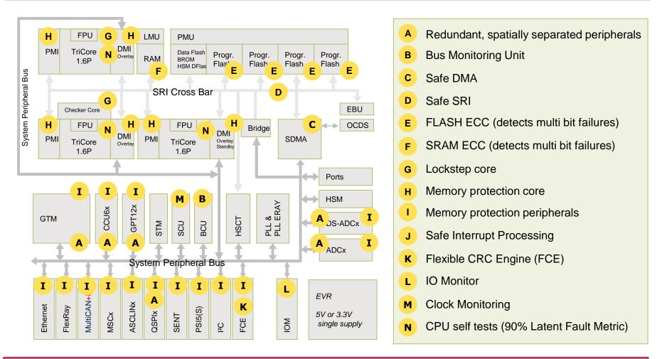
SAFETY is more than just a lockstep core. AURIX<sup>™</sup> is designed with Pro-SIL<sup>™</sup> (Safety Integrity Level) features throughout
