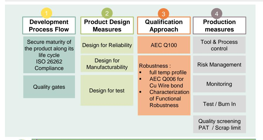
The Next Level of Zero Defect program ensures Quality throughout the Product Life Cycle, with Infineon 32-bit MCUs already reaching < 1ppm
