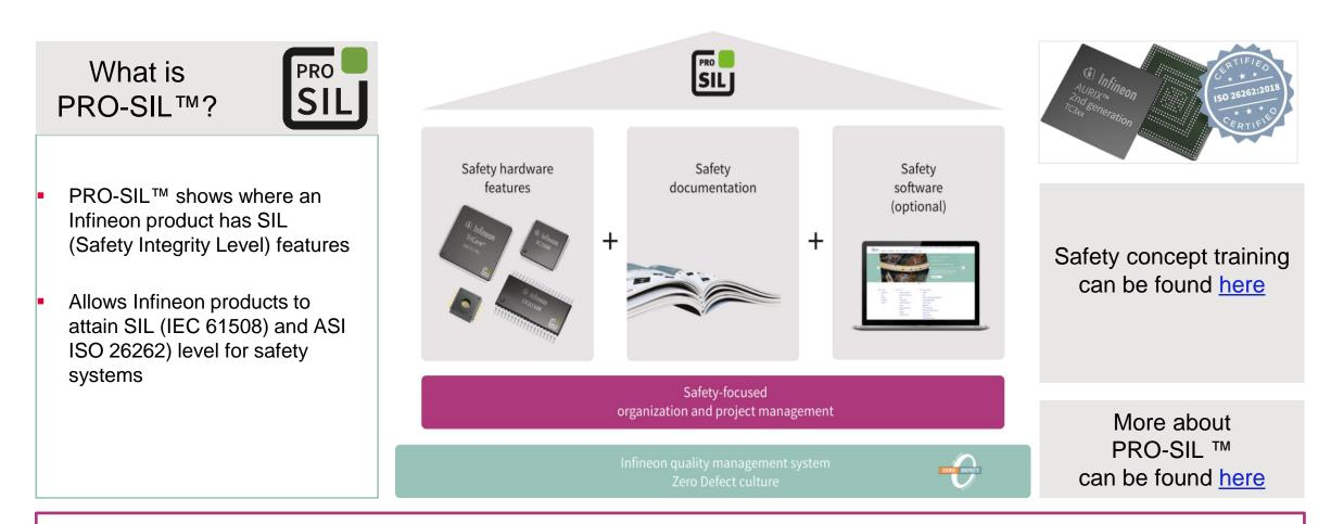
The AURIX<sup>™</sup> is PRO-SIL<sup>™</sup> compliant with safety hardware features throughout. Documentation may require an NDA. PRO-SIL<sup>™</sup> SafeTlib Safety Software is available.
