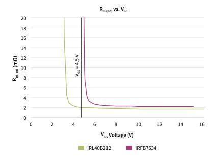
Logic level  $R_{DS(on)}$  curve vs. standard  $R_{DS(on)}$  curve
