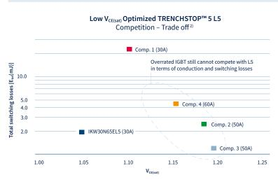
1) Datasheets value for 30A DuoPack IGBT, IKW30N65EL5 2)  $\rm T_{v_1}$  = 25°C,  $\rm I_{CE}$  = 30A,  $\rm R_g$  = 10 $\Omega$
