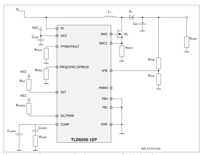
Figure 30 Constant output voltage boost converter application schematic
