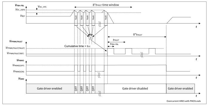
Figure 21 System behavior with R<sub>FPWM/FAULT(H)</sub> during overcurrent detection with PMOS as dimming/protection element
