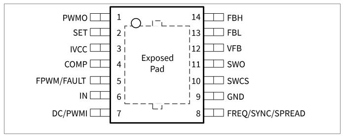
Figure 3 Pin configuration PG-TSDSO-14
