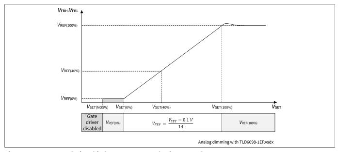
Figure 13 Relationship between  $V_{SET}$  and reference voltage  $V_{REF}$
