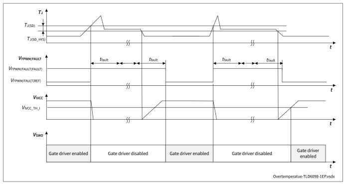
Figure 25 Timing diagram during overtemperature protection
