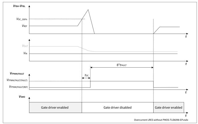
Figure 24 System behavior  $R_{\mathsf{FPWM}/\mathsf{FAULT}(\mathsf{L})}$  during overcurrent detection without PMOS as dimming/protection element
