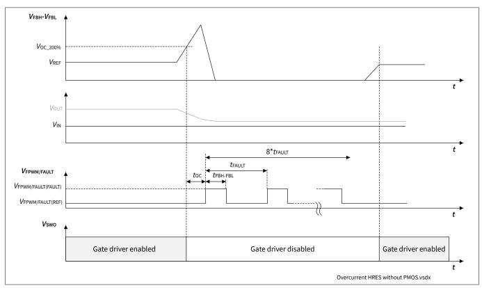
System behavior with  $R_{\text{FPWM/FAULT(H)}}$  during overcurrent detection without PMOS as Figure 22 dimming/protection element
