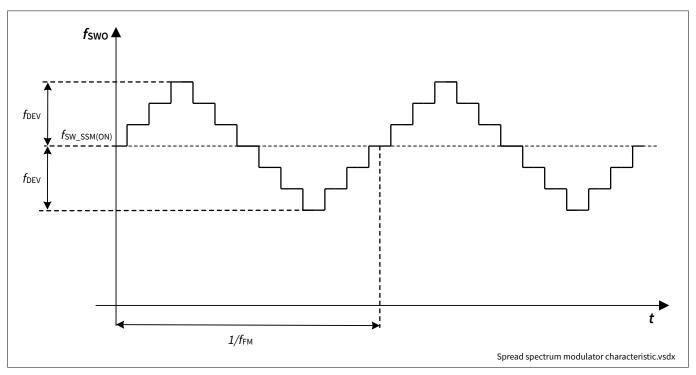
Figure 11 Spread spectrum modulator characteristic
