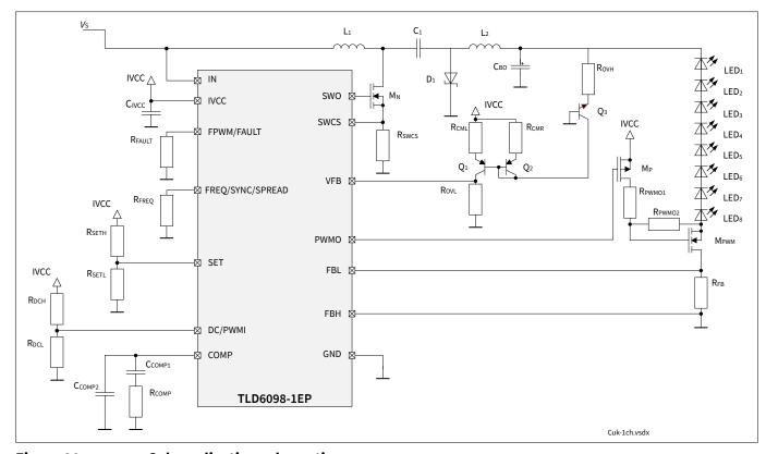
Figure 29 Cuk application schematic
