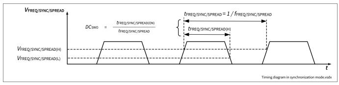
Figure 12 Timing diagram when synchronization mode is enabled
