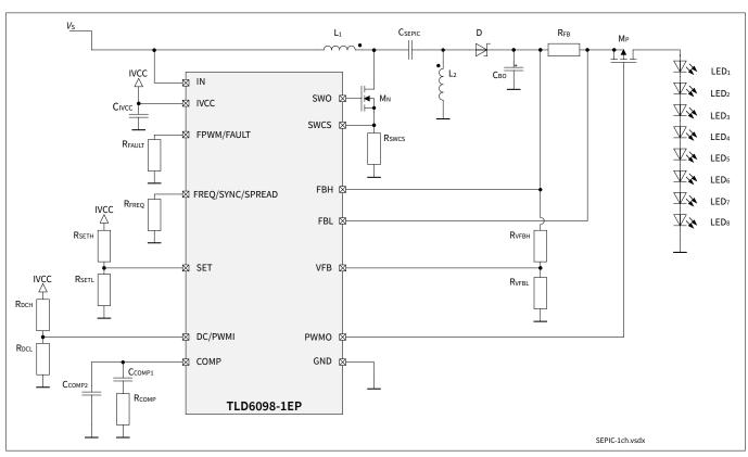
Figure 28 SEPIC application schematic
