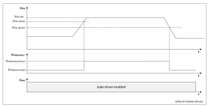
Figure 18 Timing diagram in voltage regulation
