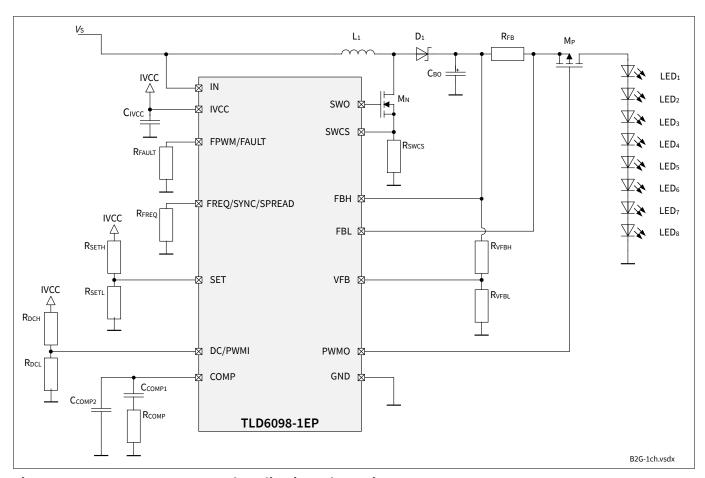
Figure 26 Boost to ground application schematic
