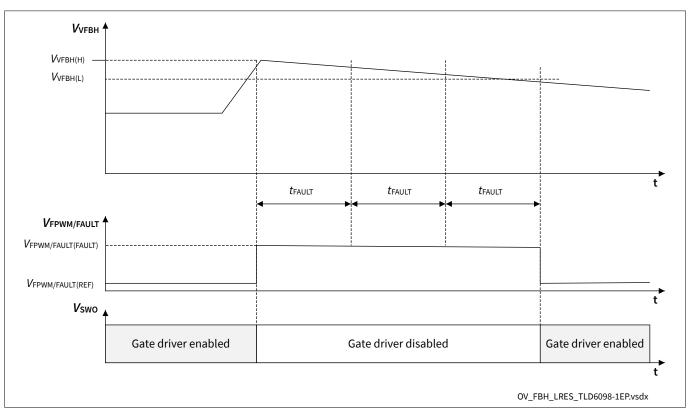
Figure 20 Timing diagram during overvoltage on FBH detection with  $R_{\text{FPWM/FAULT(L)}}$  used on FPWM/FAULT pin
