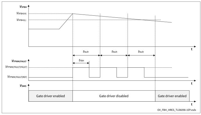
Figure 19 Timing diagram during overvoltage on FBH detection with  $R_{\text{FPWM/FAULT(H)}}$  used on FPWM/FAULT pin
