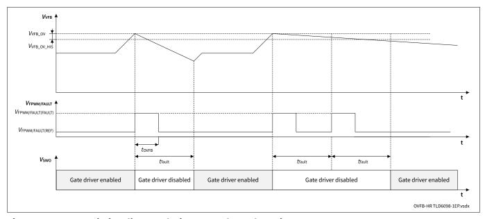
Figure 17 Timing diagram during overvoltage detection
