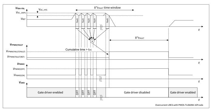
Figure 23 System behavior with R<sub>FPWM/FAULT(L)</sub> during overcurrent detection with PMOS as dimming/protection element
