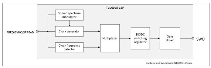
Diagram of switching frequency adjustment and synchronization blocks Figure 9
