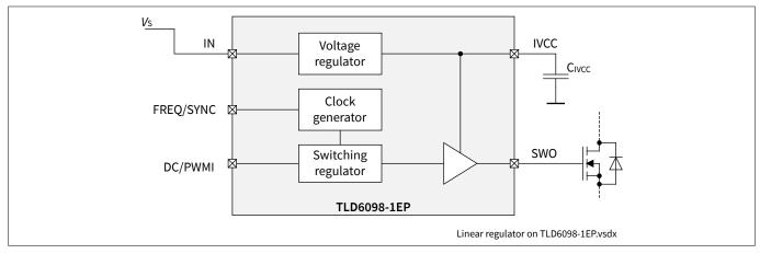
Figure 7 Block diagram of the linear regulator
