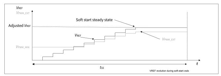
Figure 6  $V_{REF}$  and  $V_{PWM\_EXT}$  waveforms during the soft start routine with analog output adjustment
