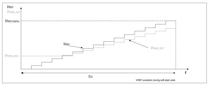
Figure 5  $V_{\text{REF}}$  and  $V_{\text{PWM\_EXT}}$  waveforms during the soft start routine without analog output adjustment
