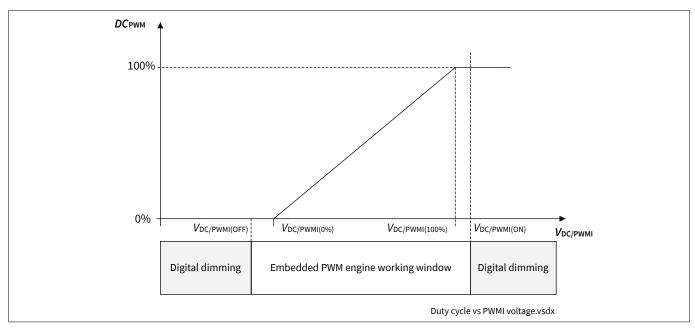
Figure 14 Relationship between V<sub>DC/PWMI</sub> and dimming duty cycle
