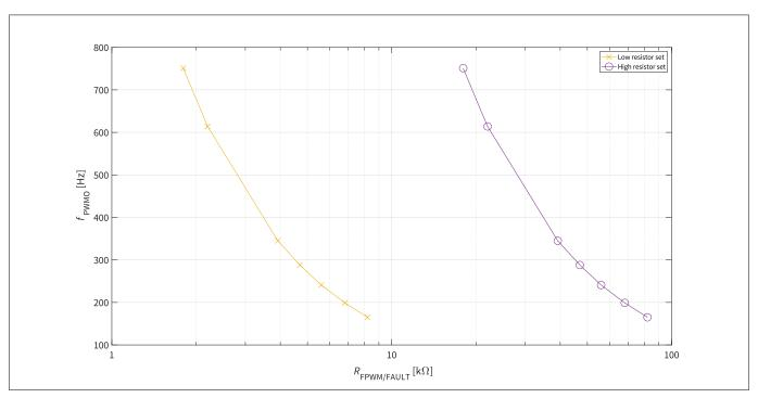
Figure 15 Relationship between  $R_{\text{FPWM/FAULT}}$  and the frequency of PWMO
