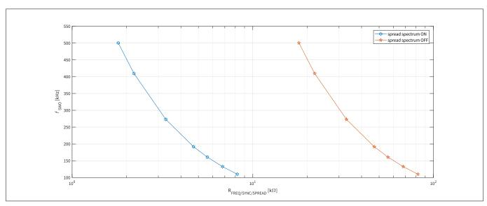
Figure 10 Switching frequency versus R<sub>FREQ/SYNC/SPREAD</sub>
