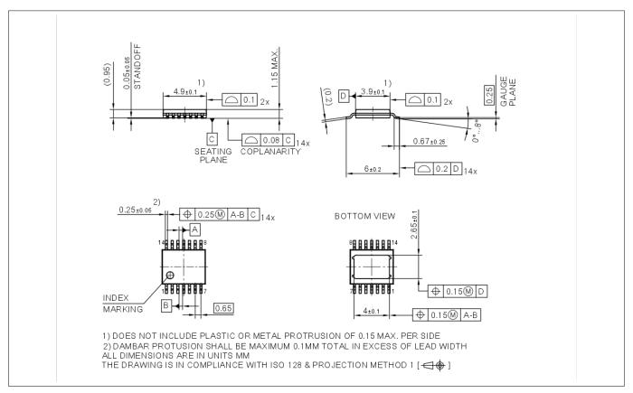
Figure 31 Package dimensions PG-TSDSO-14
