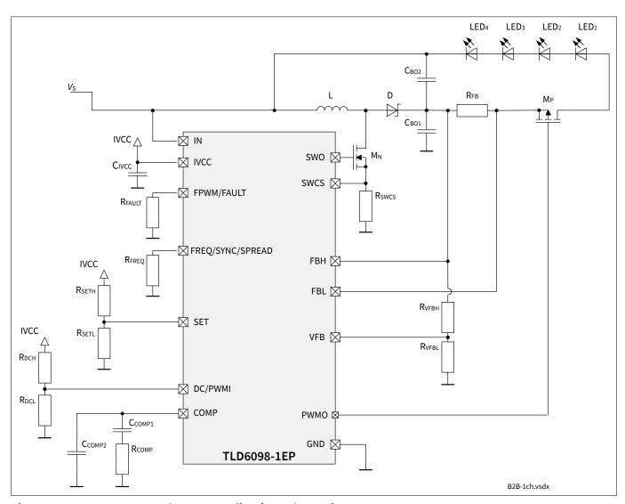
Figure 27 Boost to battery application schematic
