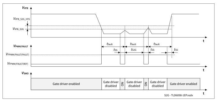
Figure 16 Timing diagram during short to ground detection
