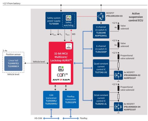
Thanks to its state-of-the-art safety features, the new TriCore™ AURIX™ family enables systems to achieve the highest ASIL-D safety level, which is already required in contemporary suspension systems.
