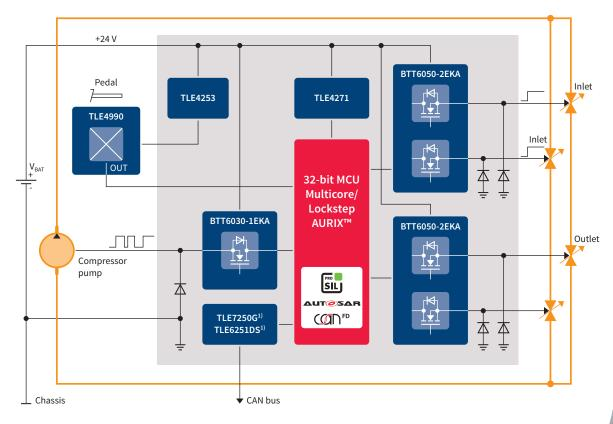
A 24 V complete system solution for hydraulic/pneumatic management systems: power supply, sensors, microcontrollers and high-side switches can be used without external protection in a 24 V system. Valves and pumps can be driven via linear activation or demand-controlled via PWM signals.
