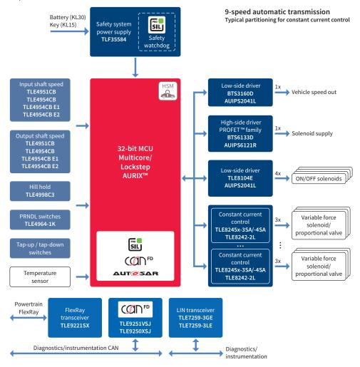
Thanks to its state-of-the-art safety features, the TriCore™ AURIX™ family enables systems to achieve the highest safety level up to ASIL-D. The rich scalability of the AURIX™ family permits a platform approach that meets the needs of a range of transmission systems. Furthermore, the hot temperature package and bare die solutions enable AURIX™ to be used in both attached and integrated control units.
