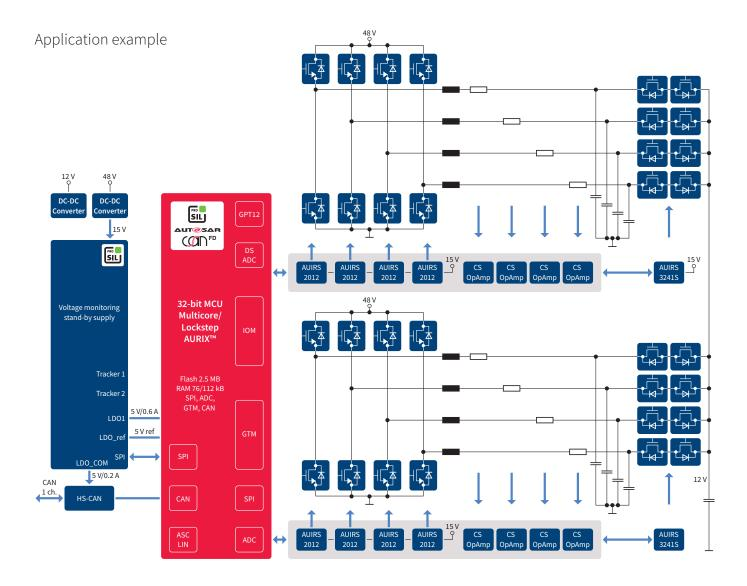
The DC-DC converter ECU is responsible for the conversion of voltage between the 48 V domain and the 12 V domain in mild hybrid cars. The 48 V domain powers stop-start motors, hybrid motors, and turbochargers, enabling engine downsizing and better fuel economy and performance.
