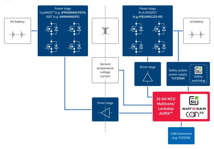
The DC-DC converter ECU is responsible for the conversion of voltage between the main battery of the car, that is, the high voltage battery to the 12 V domain in full hybrid, plug-in hybrid and electrical vehicles.
