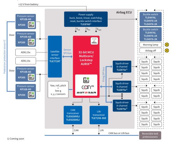
Thanks to its state-of-the-art safety features, the new TriCore™ AURIX™ family enables systems to achieve the highest safety level up to ASIL-D.
