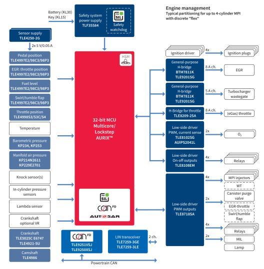
Thanks to its state-of-the-art safety features, the TriCore™ AURIX™ family enables systems to achieve the highest safety level up to ASIL-D. The scalable AURIX™ family includes the GTM, the de-facto industry standard timing module that supports highly complex engine management, while meeting the market's most stringent emissions regulations.
