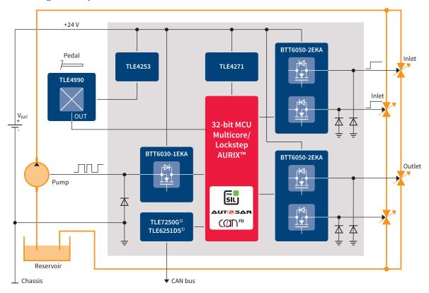
1) If ECU permanently supplied, you may need to add external protection against load dump 400 ms above 40 V.
