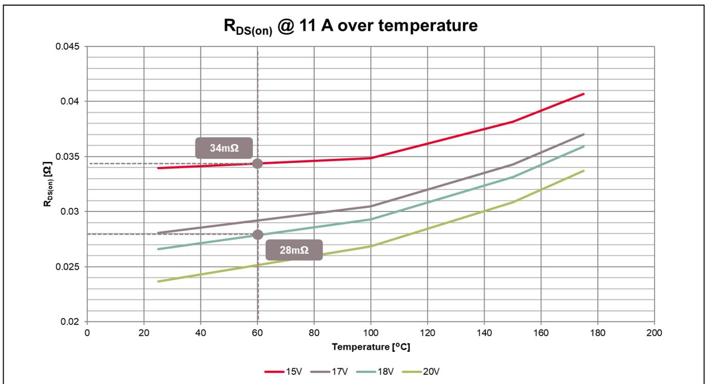
Figure 16  $R_{DS(on)}$  dependency on  $V_{GS}$
