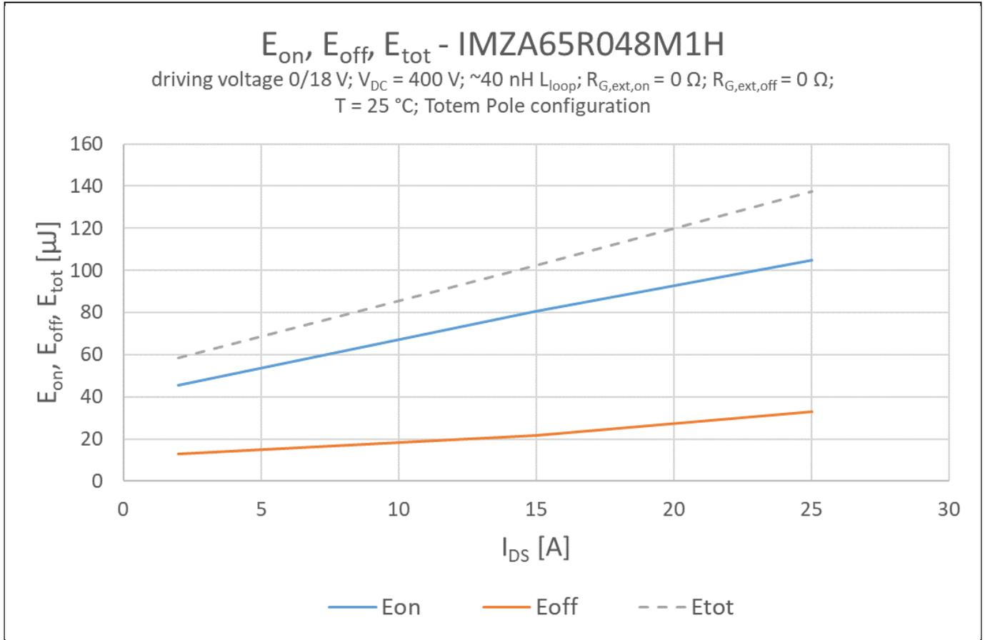
Figure 24 Typical switching energies for IMZA65R048M1H
