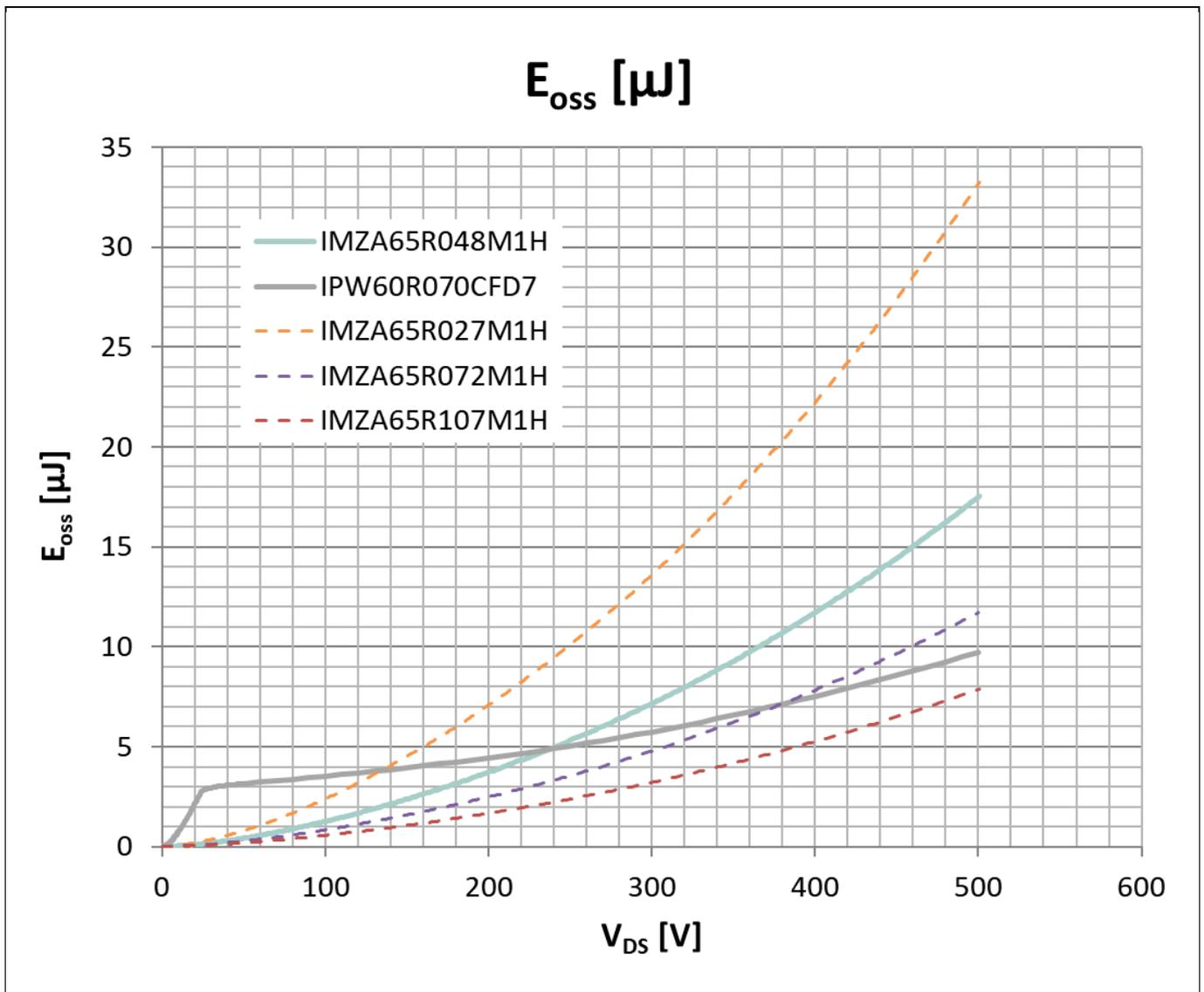
**Figure 13**  $E_{oss}$  comparison between CoolMOS™ and CoolSiC™
