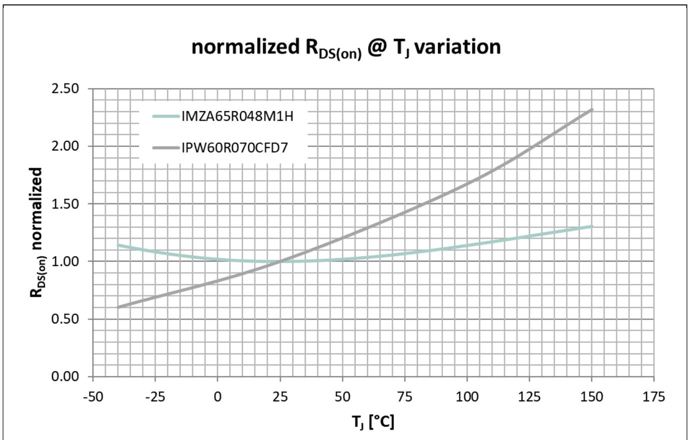
Figure 6 Normalized R<sub>DS(on)</sub> over-temperature comparison between CoolMOS™ and CoolSiC™
