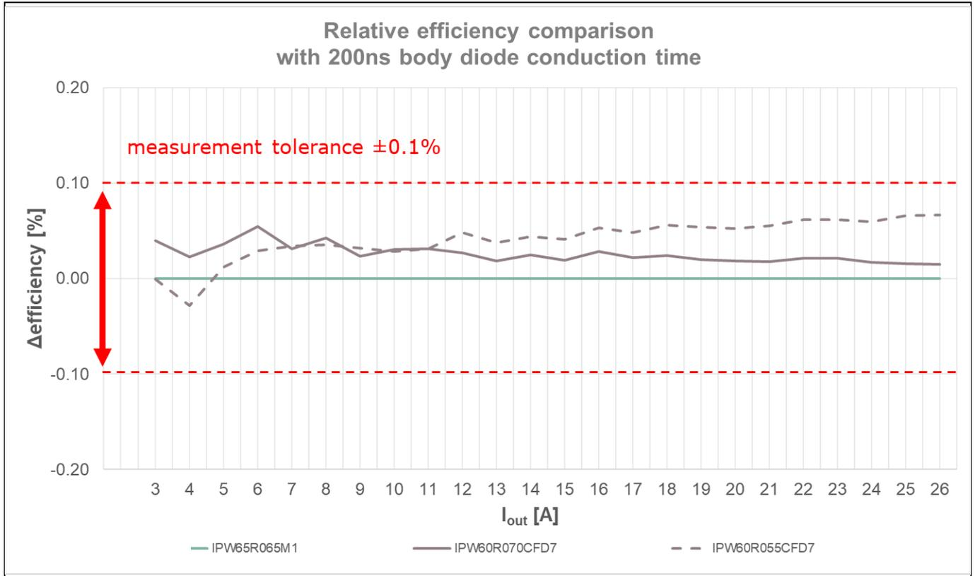
**Figure 30 Relative efficiency comparison with 200 ns body diode conduction time**
