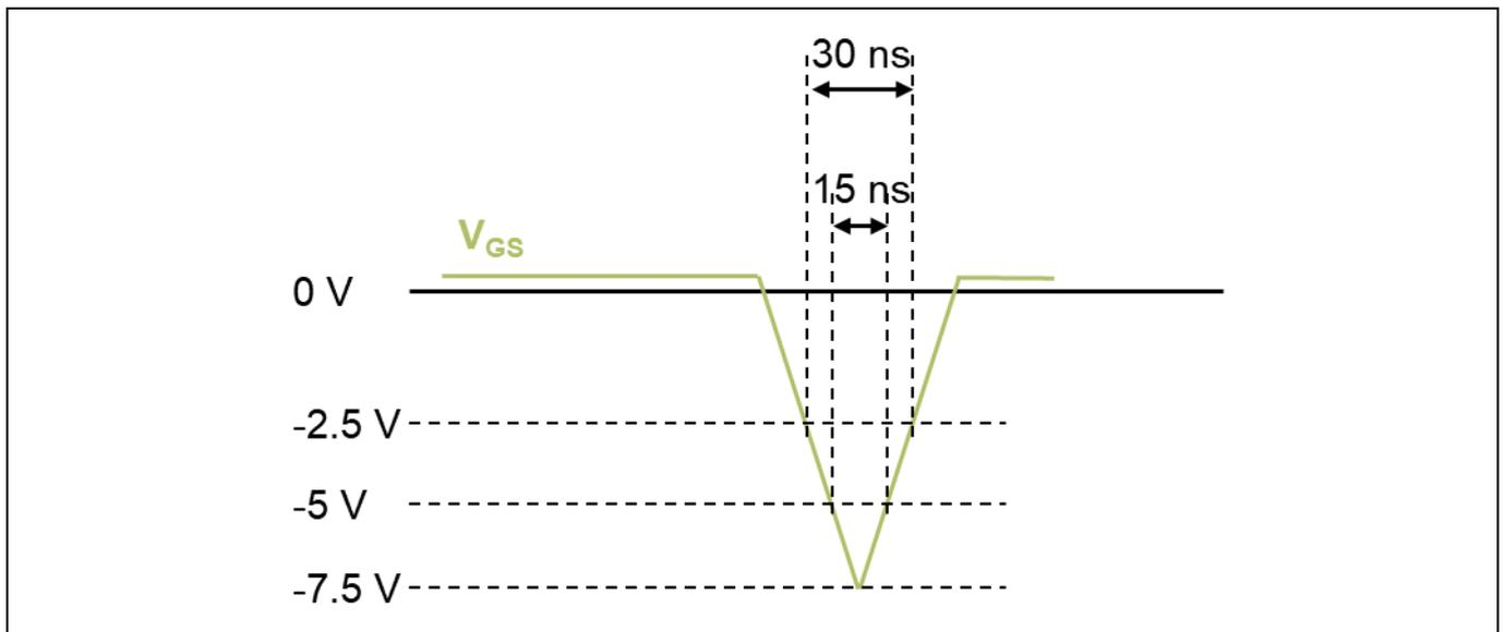
Figure 18 Test parameters to see the impact of negative  $V_{GS}$  in the CCM totem pole PFC
