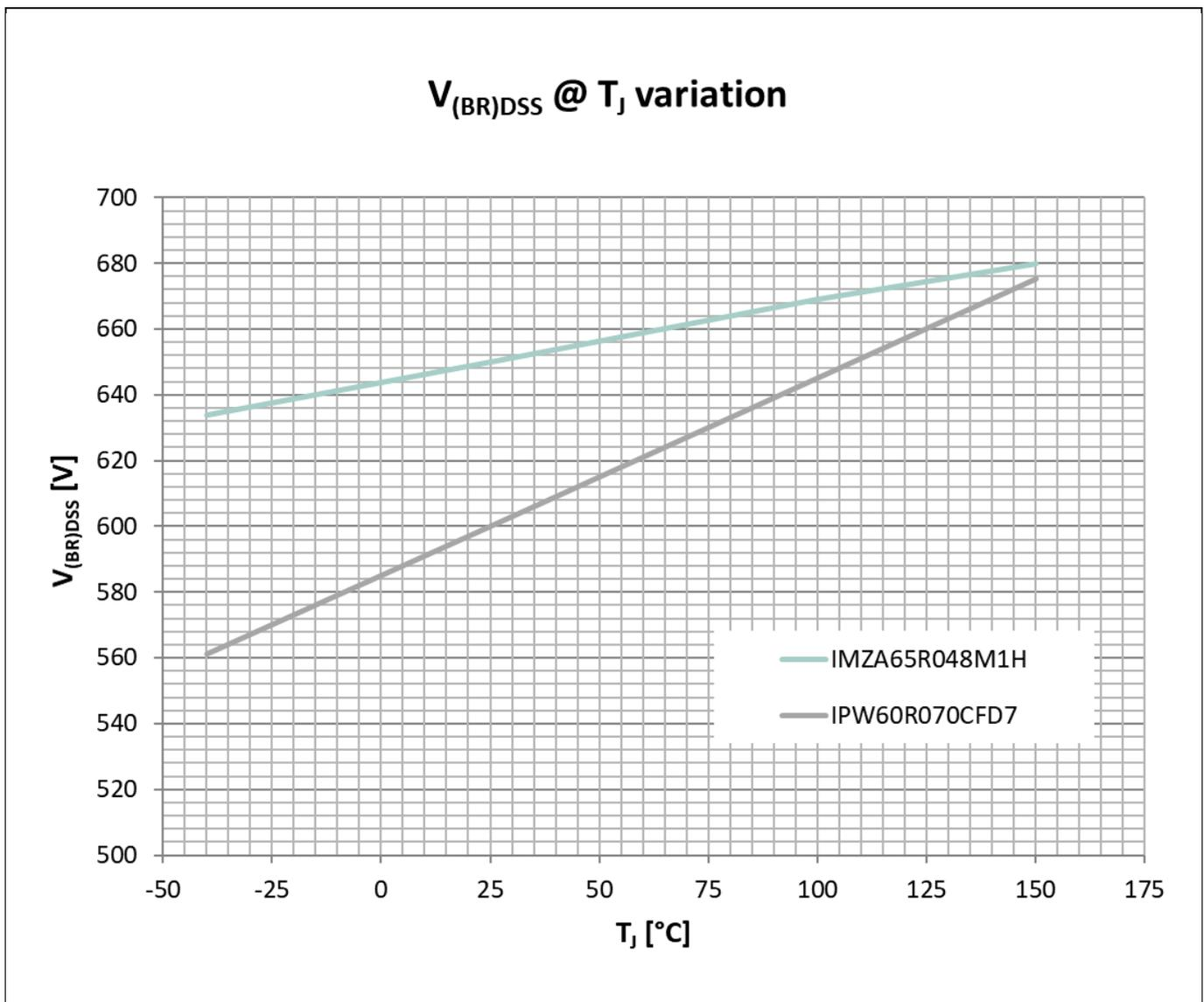
Figure 9  $V_{(BR)DSS}$  comparison between CoolMOS™ and CoolSiC™
