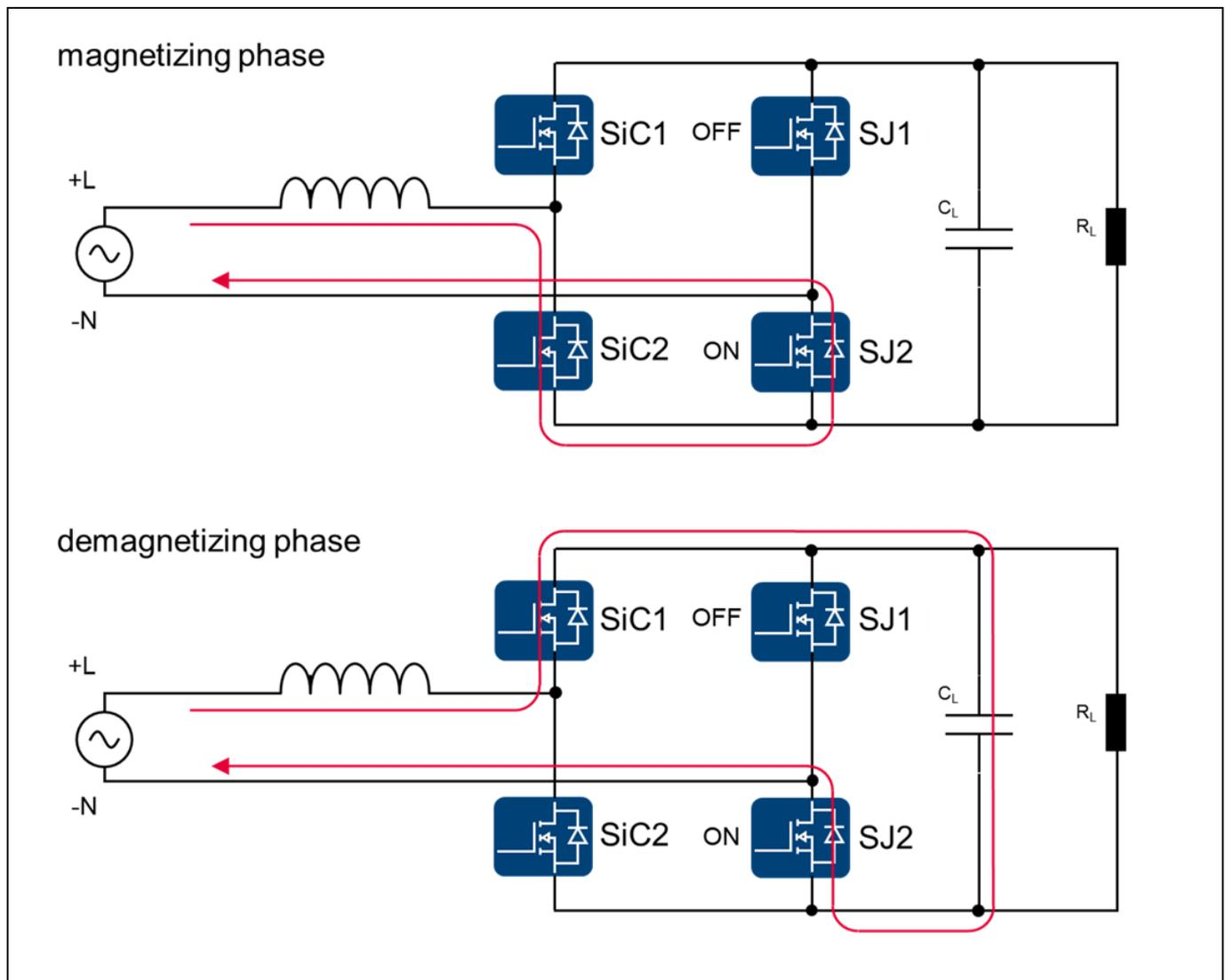
Figure 4 Operating principle of positive AC-line cycle
