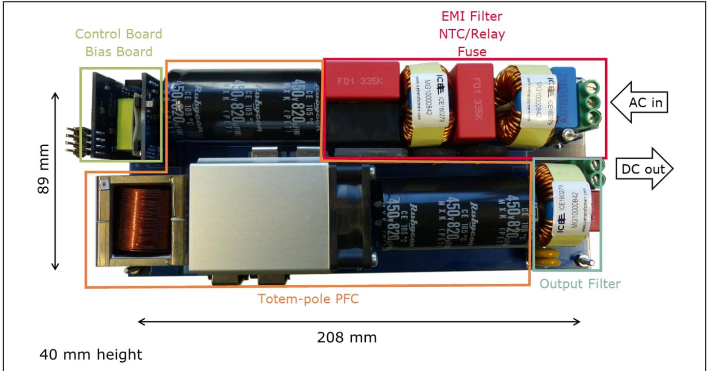
**Figure 26 3.3 kW CCM totem pole PFC**
