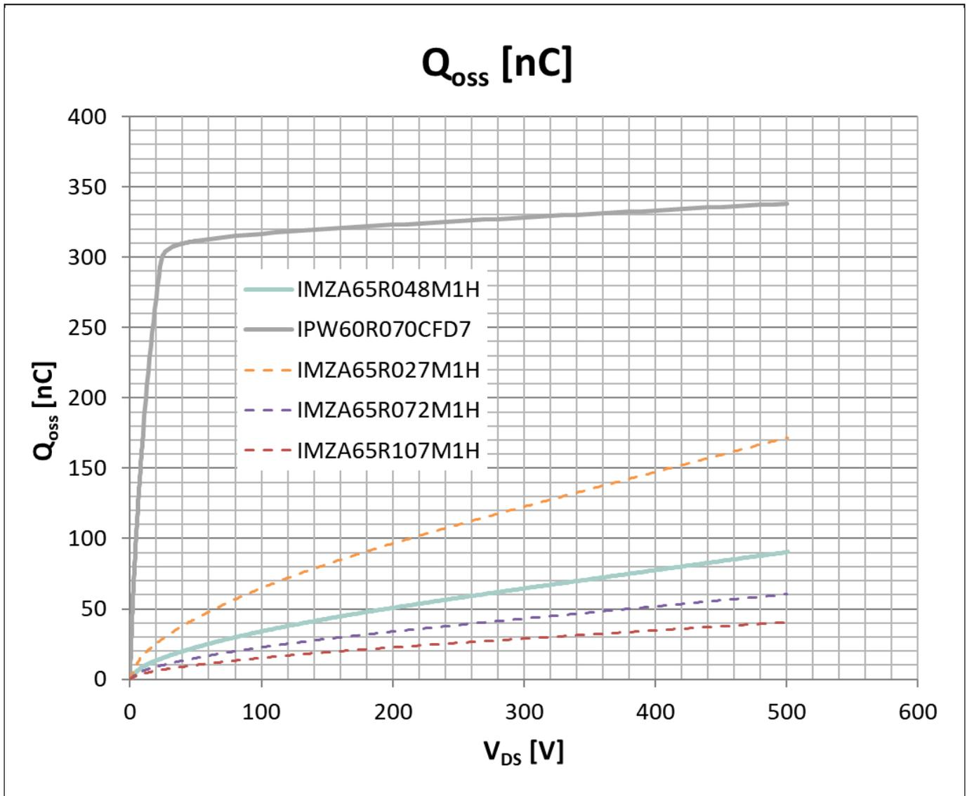
**Figure 14** **Q<sub>oss</sub> comparison between CoolMOS™ and CoolSiC™**
