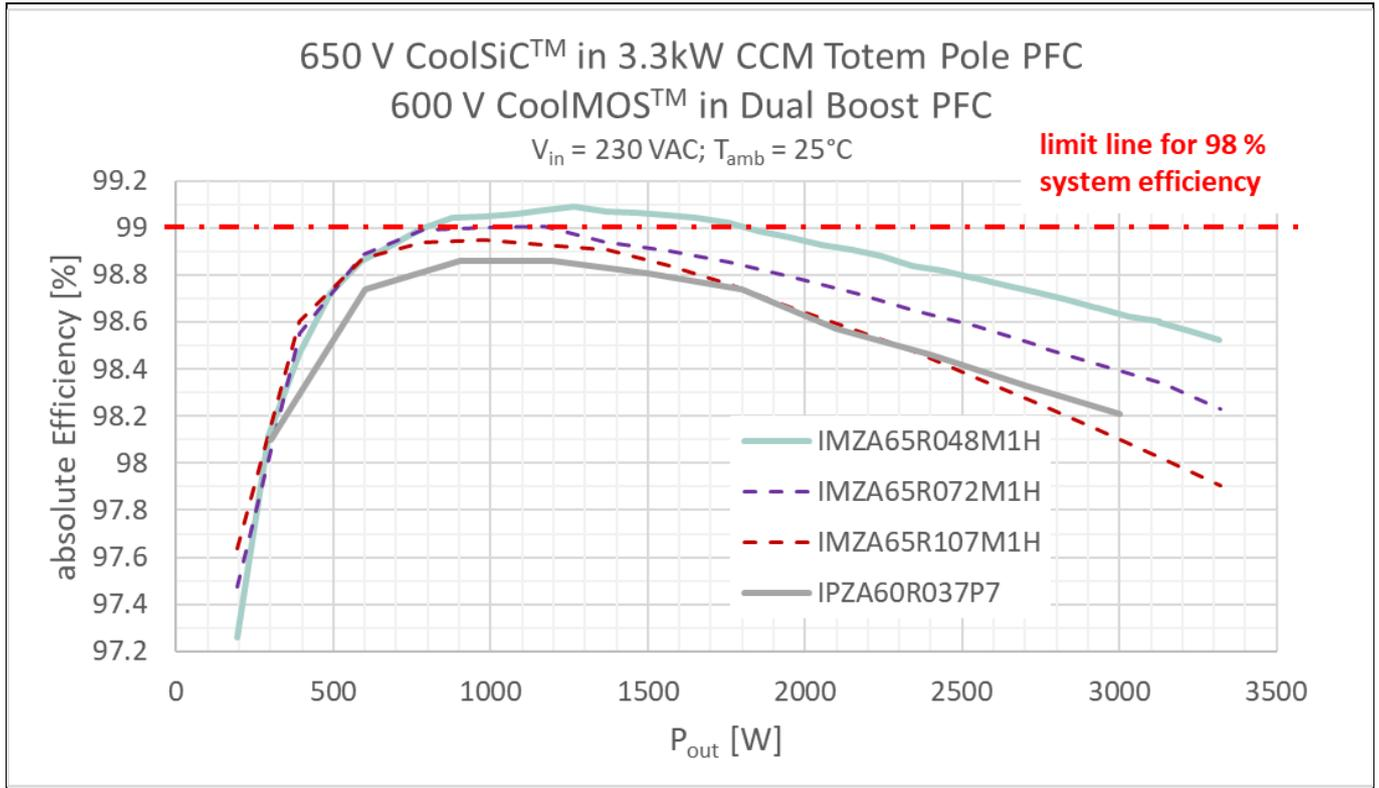
**Figure 27 Efficiency comparison between CoolMOS™ and CoolSiC™**
