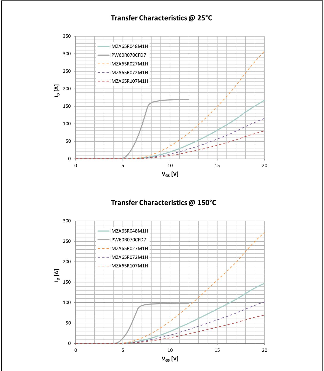
Figure 10 Transfer characteristics comparison between CoolMOS™ and CoolSiC™ at V<sub>DS</sub> = 20 V; T<sub>J</sub> = 25°C (upper) and T<sub>J</sub> = 150°C (lower)
