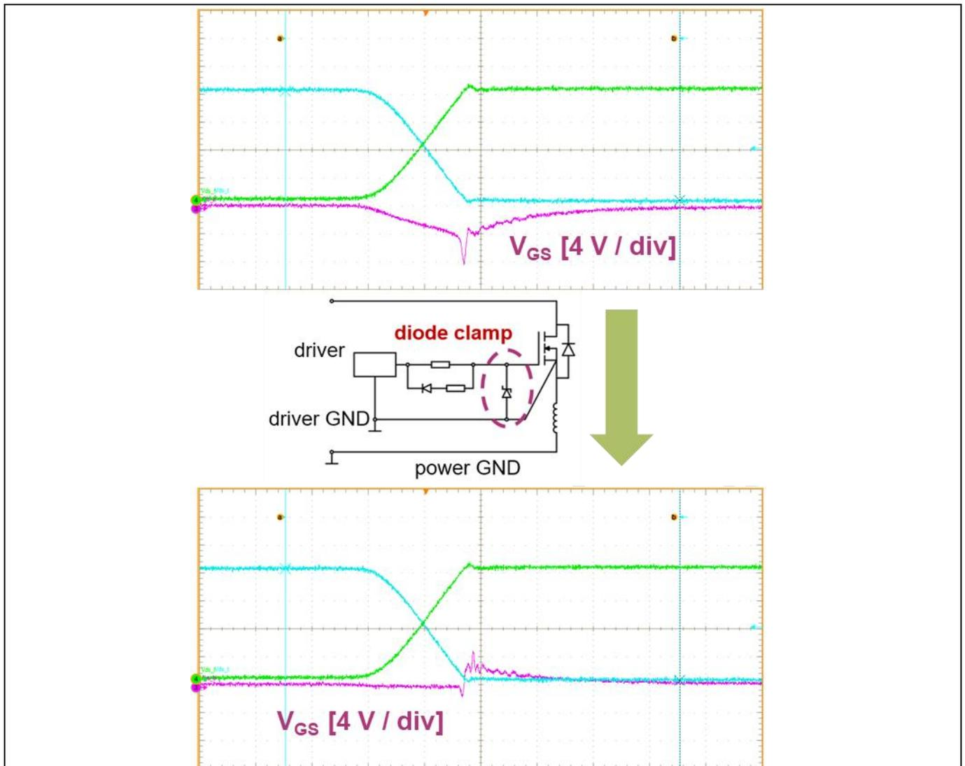
Figure 19 Impact of diode clamp
