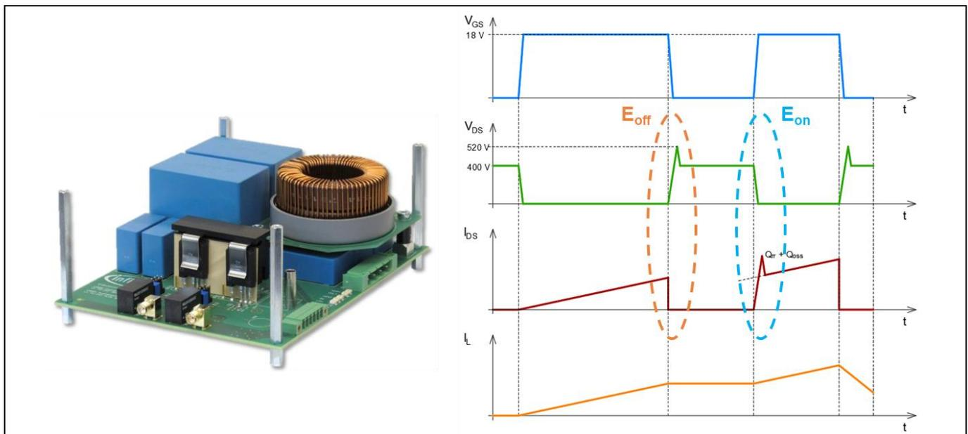
**Figure 22 Test set-up for  $E_{on}$  and  $E_{off}$  measurements (double-pulse set-up)**
