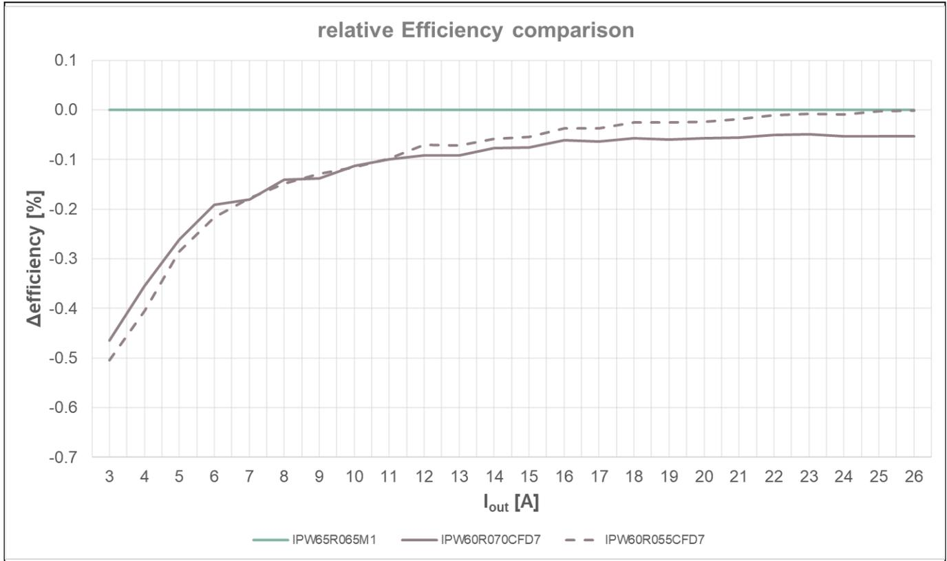
**Figure 29 Relative efficiency comparison with optimized body diode conduction time**
