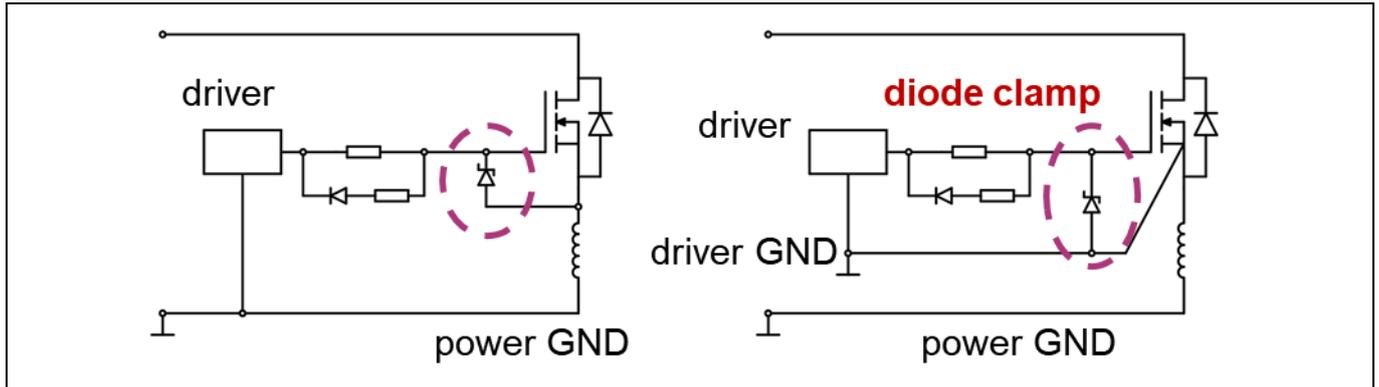
**Figure 20 Diode clamp recommendation for standard and Kelvin source connection**
