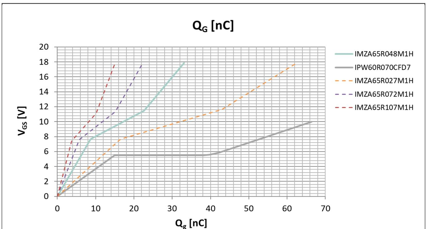
**Figure 15  $Q_G$  comparison between CoolMOS™ and CoolSiC™**
