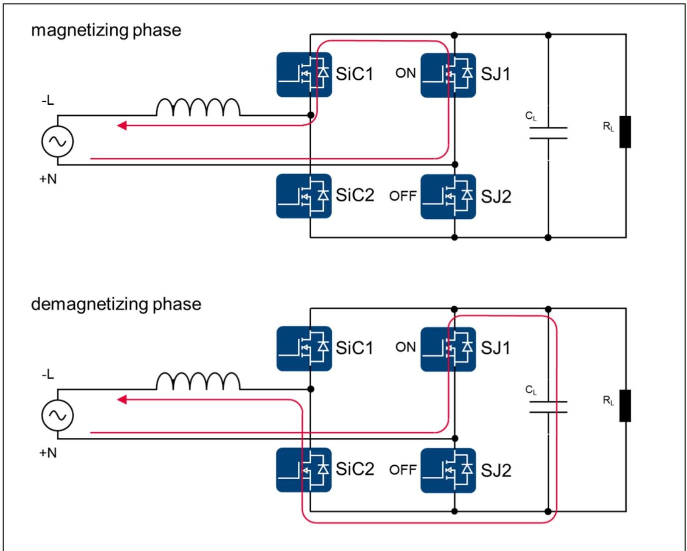
Figure 5 Operating principle of negative AC-line cycle
