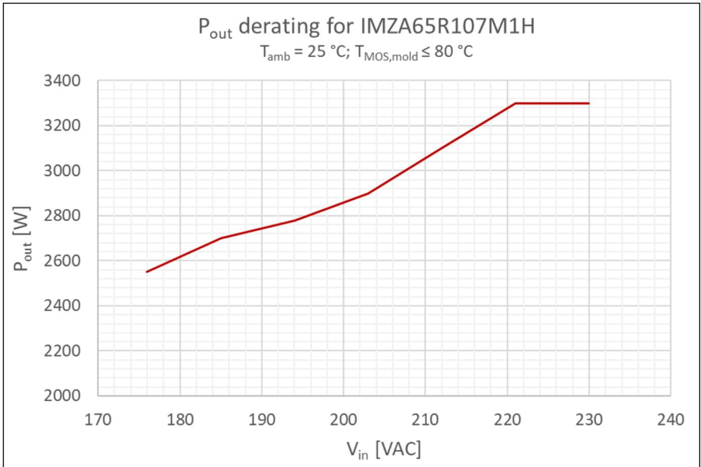
**Figure 28 Power de-rating need for low  $V_{in}$  for IMZA65R107M1H**
