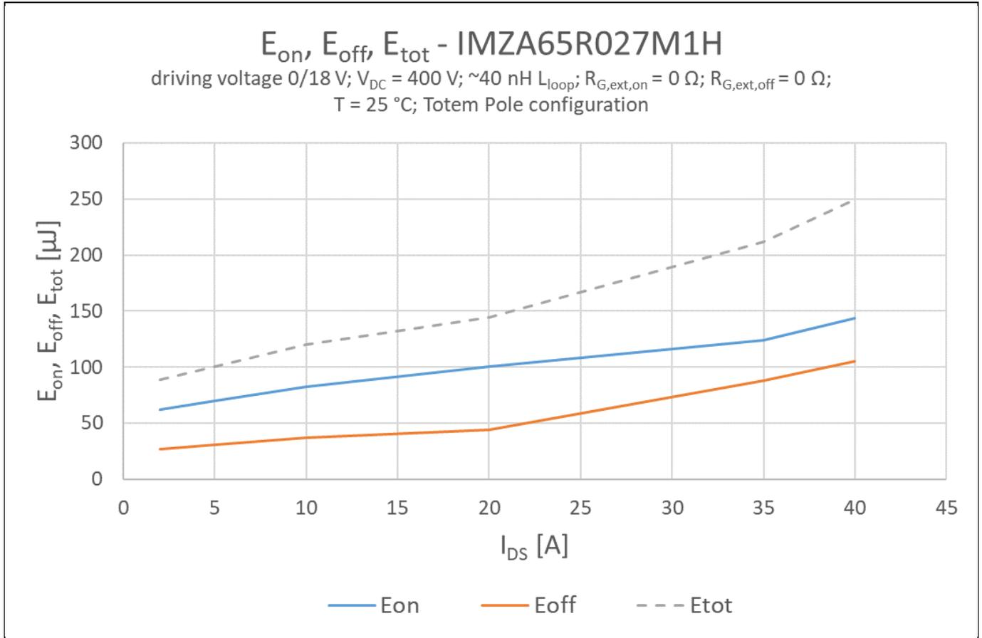
Figure 23 Typical switching energies for IMZA65R027M1H
