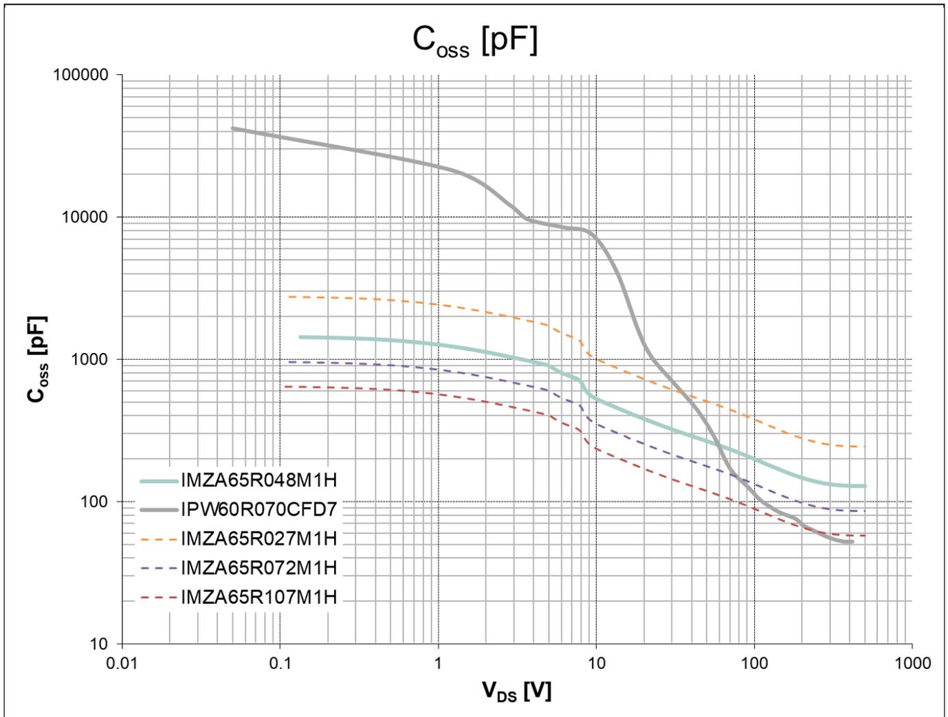
Figure 11 Typical C<sub>oss</sub> of CoolMOS™ and CoolSiC™
