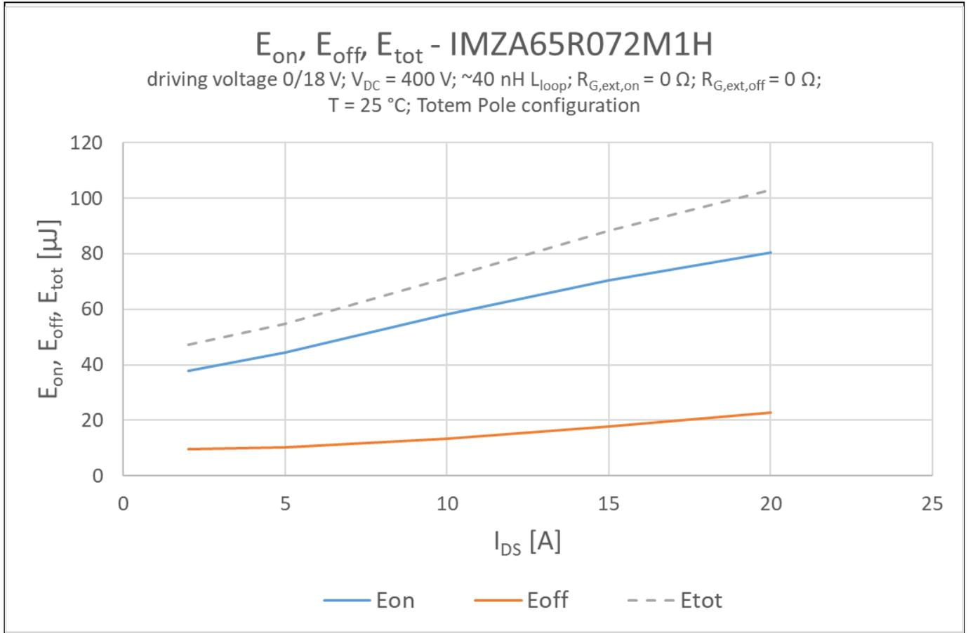
**Figure 25** Typical switching energies for IMZA65R072M1H
