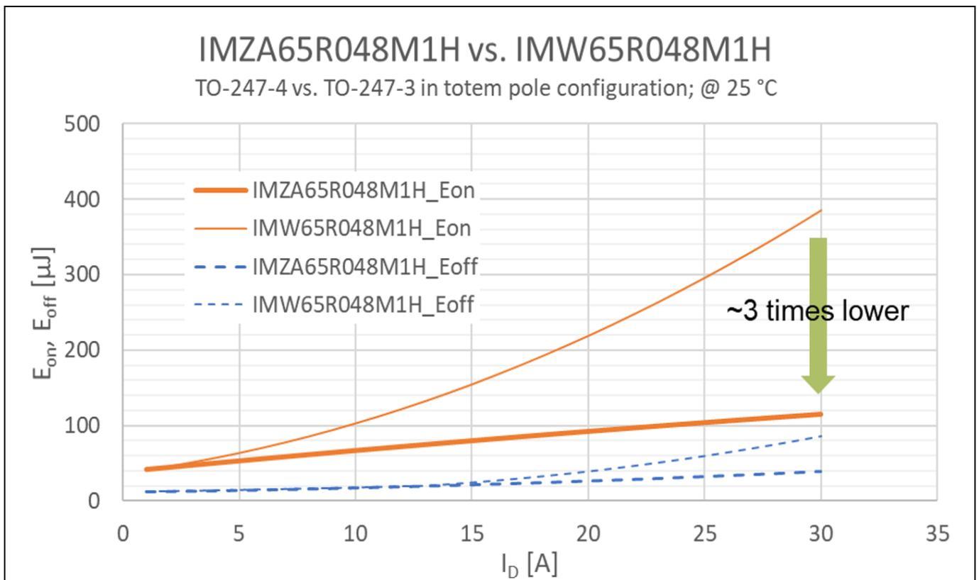
**Figure 21 Comparison of switching energies of standard and Kelvin source configuration**
