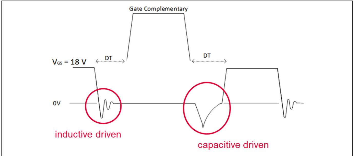
Figure 17 Root causes of negative  $V_{GS}$
