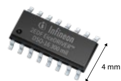
DSO16 pin Narrow body 1.27 mm lead pitch
