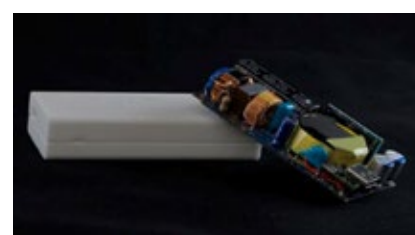
Infineon's 20 W/in 3 adapter (cased) - 24 W/in 3 (uncased) with 65 W output power capability (LxWxH: 74.2 mm x 36.5 mm x 16.5 mm)
