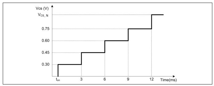
Figure 6 Maximum current sense voltage during soft start
