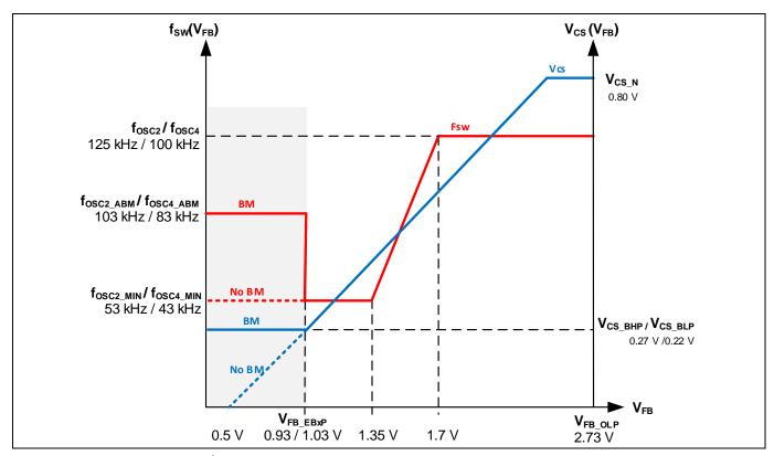
Figure 8 Frequency reduction curve
