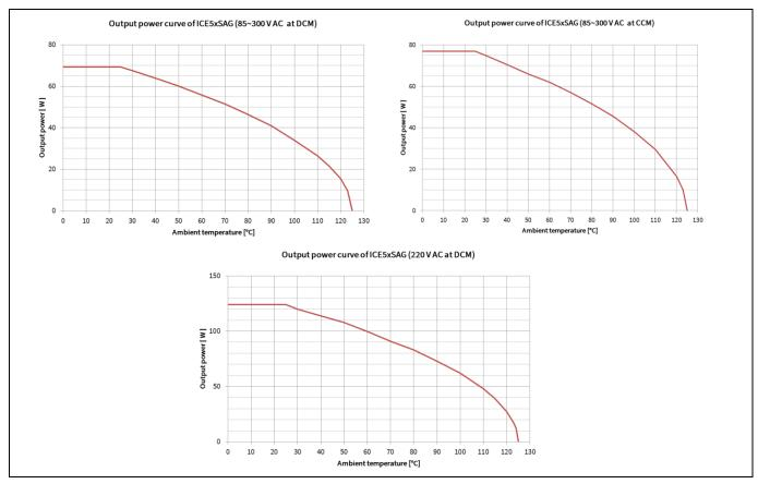
Figure 17 Output power curve of ICE5xSAG
