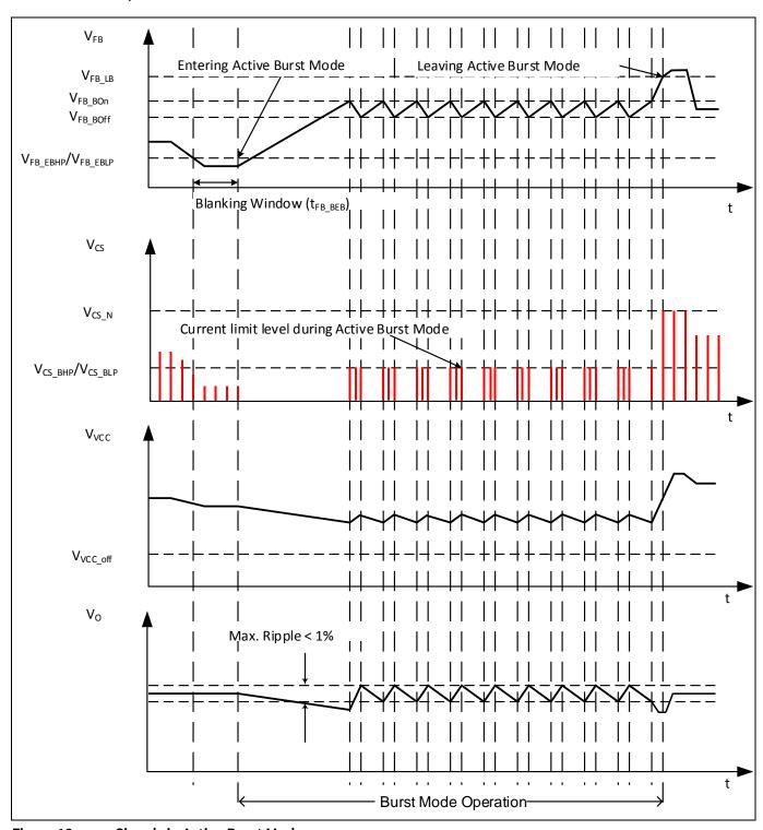
Figure 12 Signals in Active Burst Mode
