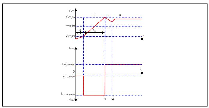
Figure 5 V<sub>cc</sub> voltage and current at startup
