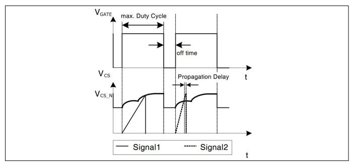
Figure 11 Dynamic voltage threshold V<sub>CS\_N</sub>
