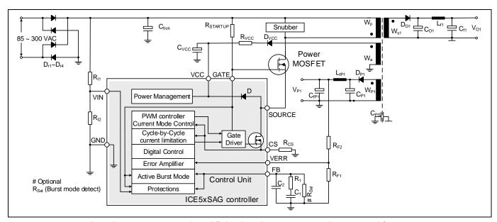
Figure 2 Typical application in non-isolated flyback utilizing integrated error amplifier
