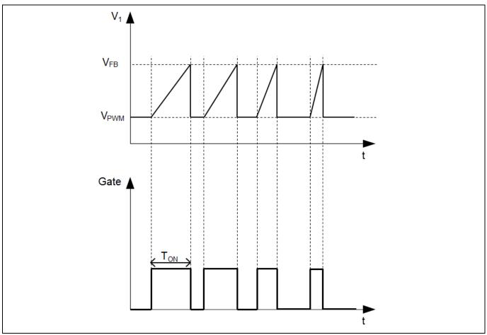
Figure 7 Pulse width modulation
