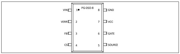
Figure 3 Pin configuration
