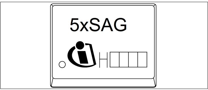
Figure 19 Marking of PG-DSO-8
