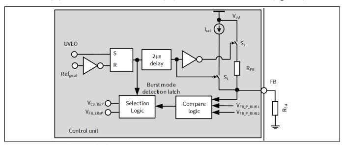
Figure 13 ABM detect and adjust
