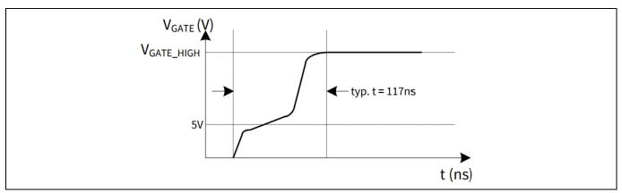
Figure 9 Gate rising waveform
