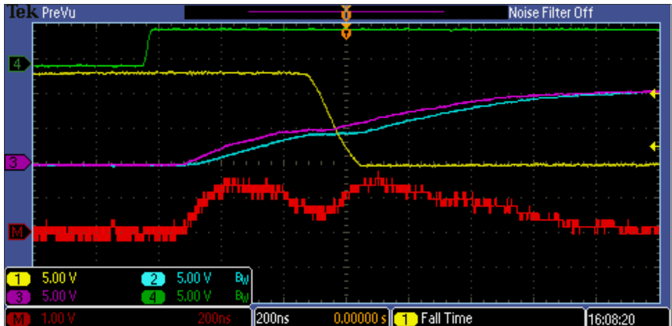
Figure 8 Turn-On Slew Rate Sequencer
