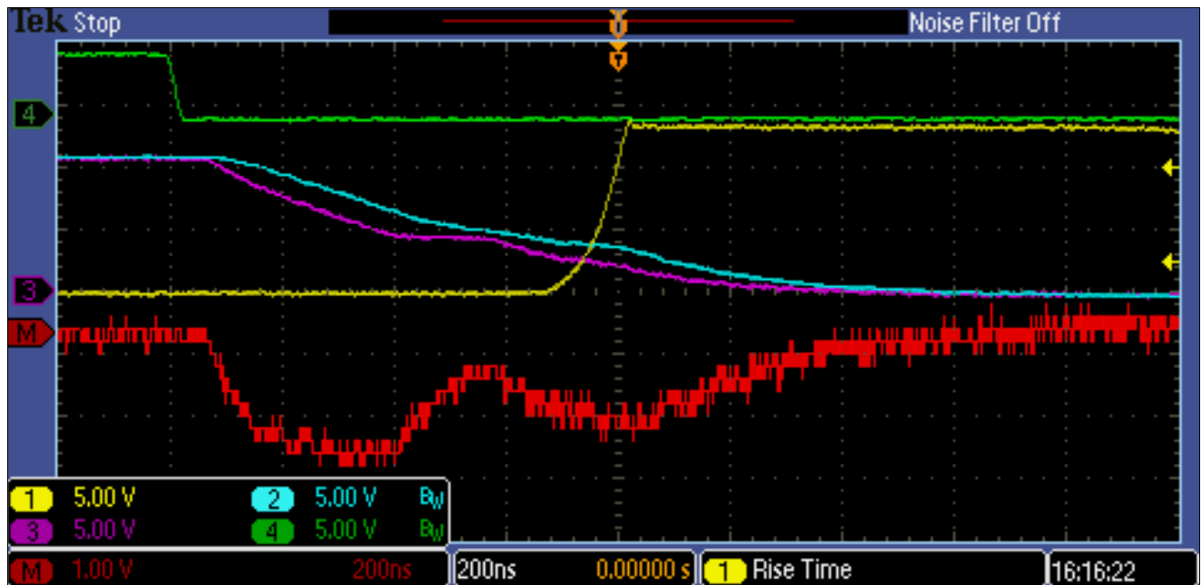
Figure 9 Turn-Off Slew Rate Sequencer
