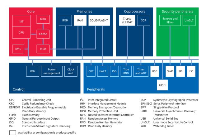
SLI 97 provides multiple interfaces and hardware crypto coprocessors, making it a perfect solution for security-critical embedded SIM (eSIM).
