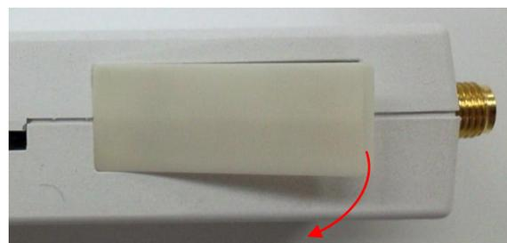
Rotate the SIM cover by 90 degrees from the direction of lifting to expose the SIM socket.
