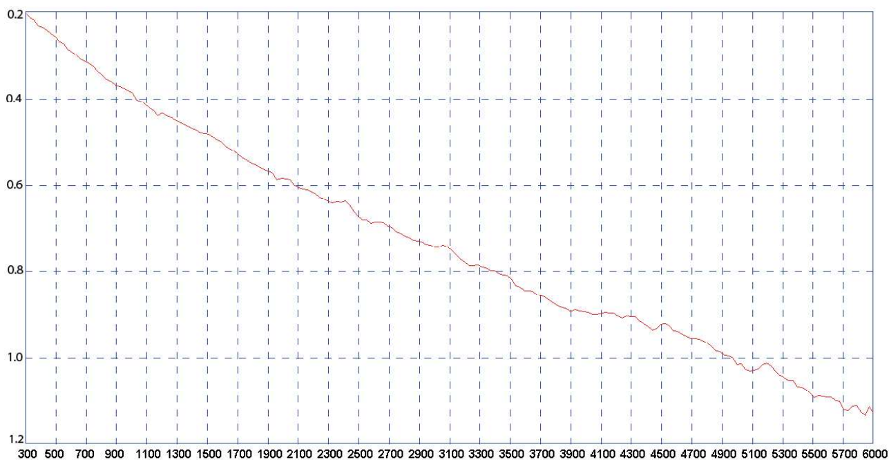
Typical Attenuation dB per m of Cable*
